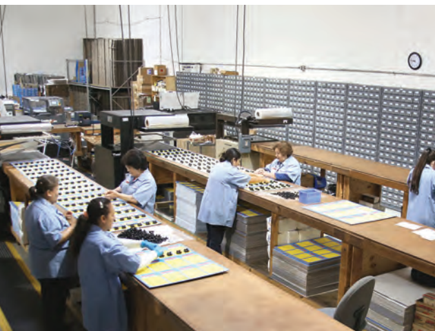
Components for each kit are placed on the appropriate display cards, sealed and labeled. Through-put has been significantly increased.
